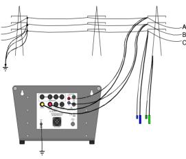
Phase A to phase B impedance test
