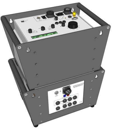
The PCU1-C is a cable impedance test system for the measurement of impedance of overhead lines and underground cables. The system consists of a separate control unit containing all metering and control functions and an output transformer that provides isolation of the output current and feedback voltage.
