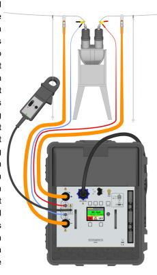
Accurate measurements on circuit breakers, isolators and grounding links with both sides earthed are simple with the optional current clamp. This allows the current flowing through the earthing equipment to be subtracted from the test current.
